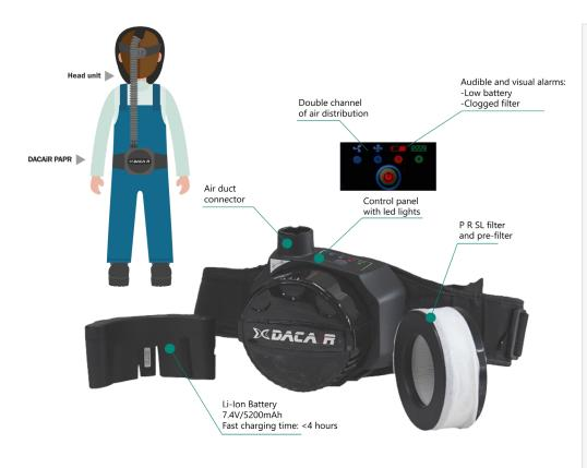
DACAiR assemblies are certified in accordance with current european legislation 425/2016 according to EN 12941:1998 + A1:2003 + A2:2008 in class TH2 or TH3 depending on the head unit Compatible with different head units, the DACAiR Powered Air Purifying Respirator (PAPR) is the most effective and versatile option to protect yourself from harmful particles in the form of dust, fumes or mists produced during welding and related techniques.
